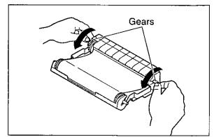
**5** Turn the film cartridge over so that the "BACK" is facing up.
